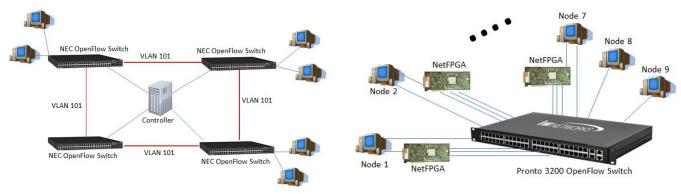
Fig. 6. Topology of the ANI OpenFlow testbed.
