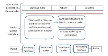
Fig. 2. Elements of an OpenFlow-compliant switch.
