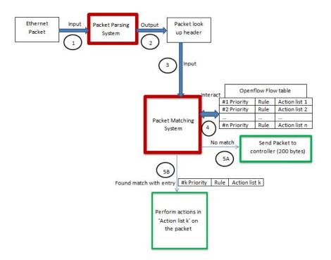
Fig. 3. How a packet is processed and forwarded in an OpenFlow 1.0.0 switch.
