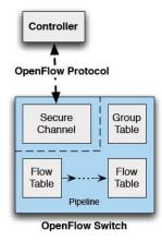
Fig. 4. Components of an OpenFlow 1.1.0 switch. Source: [18].
